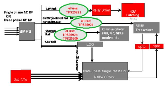
Figure 4. Proposed SMPS scheme in a smart meter
