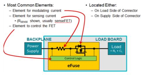
Figure 5. eFuse Block Diagram
