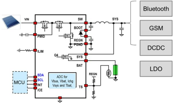
Figure 3. Example of a Flexible Charging Solution
