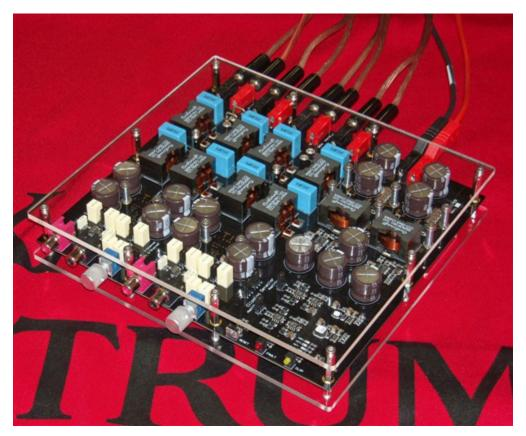
Figure 1. Built and Tested Automotive Audio Amplifier System
