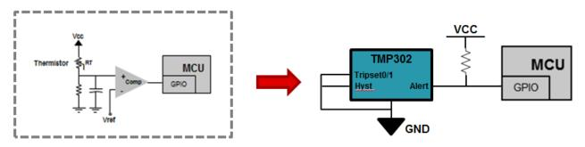
Figure 2. Temperature Switch IC vs. Discrete Temperature Switch
