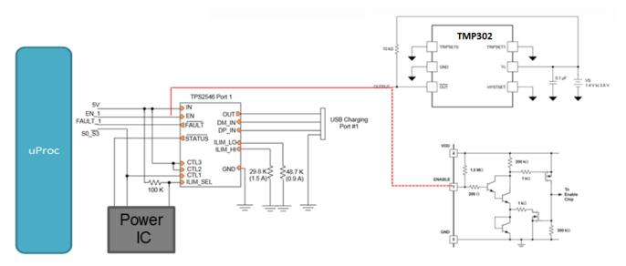
Figure 3. USB Overtemperature Protection without an MCU
