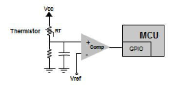
Figure 1. Thermistor and Comparator Temperature Circuit
