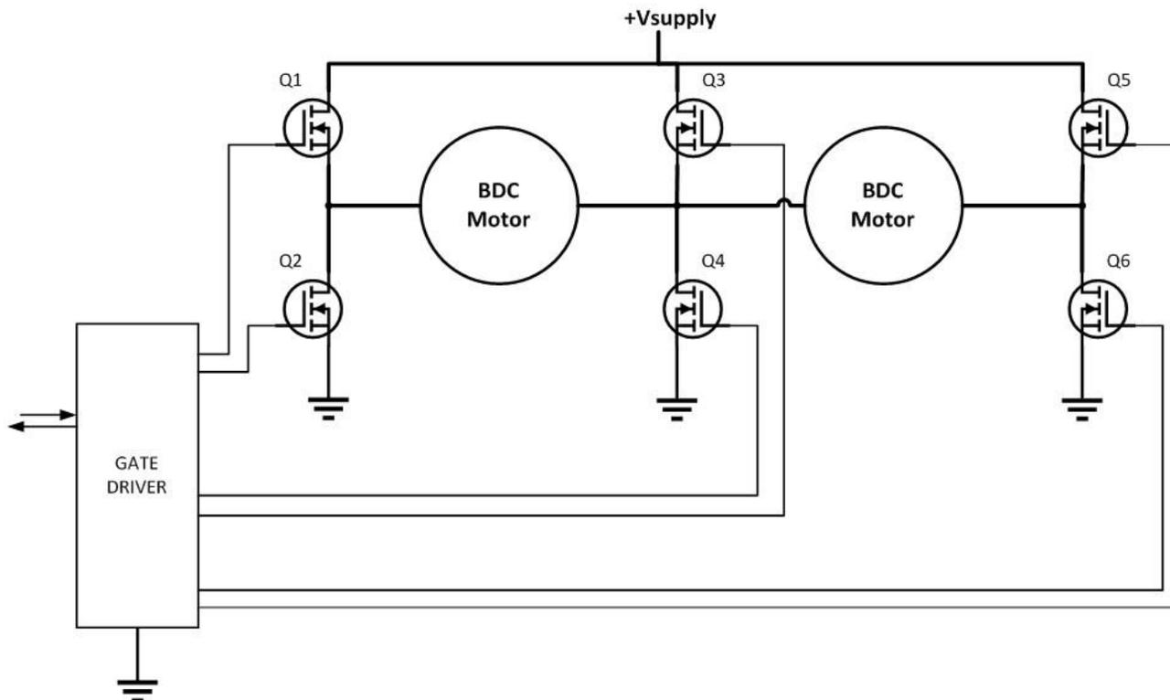
**Figure 2. Sharing MOSFETs between Motors Simplifies Seat Motor Driver Electronics**
