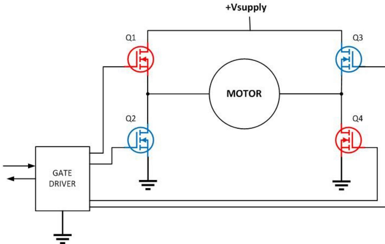
**Figure 1. H-bridge Configuration of Transistors to Enable Bidirectional Motor Rotation**
