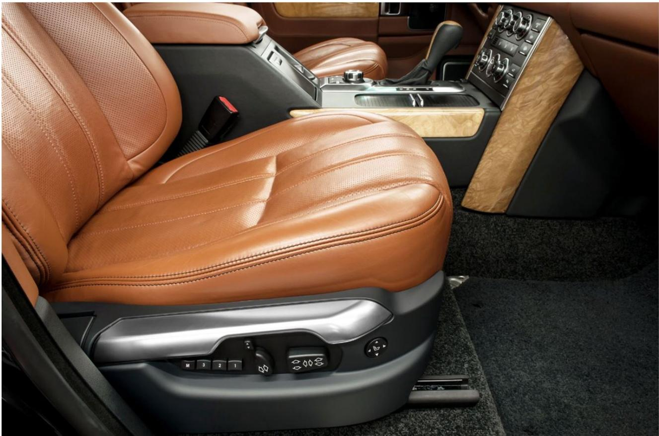
In addition, modern power seats provide the ability to adjust every aspect of the seat – distance from the steering wheel, seat height, seat tilt, lumbar support – in order for the occupant to feel comfortable. They may provide a heated or cooled cushion and back massage to enhance comfort. Seats can even rumble to the beat of the
