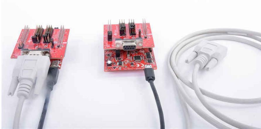
**Figure 2. RS-232 Transceiver BoosterPack™ Kit Prototype Set-up**
