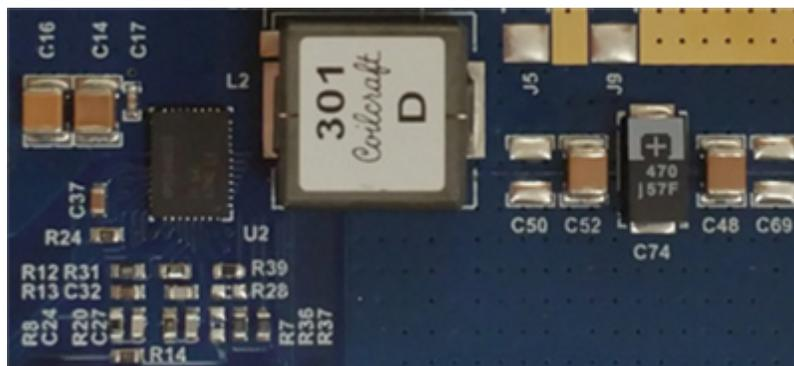
**Figure 2. The 4.5V-18V, 35A TPS546C23 PMBus Stackable Synchronous Buck Converter**
