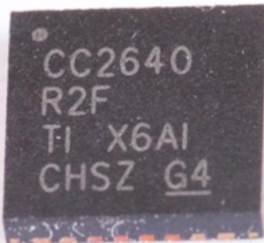
*Tiny chip goes a long way: The CC2640R2F wireless MCU comes in several package options including a 2.7mm x 2.7mm chip-scale package (WCSP)*
