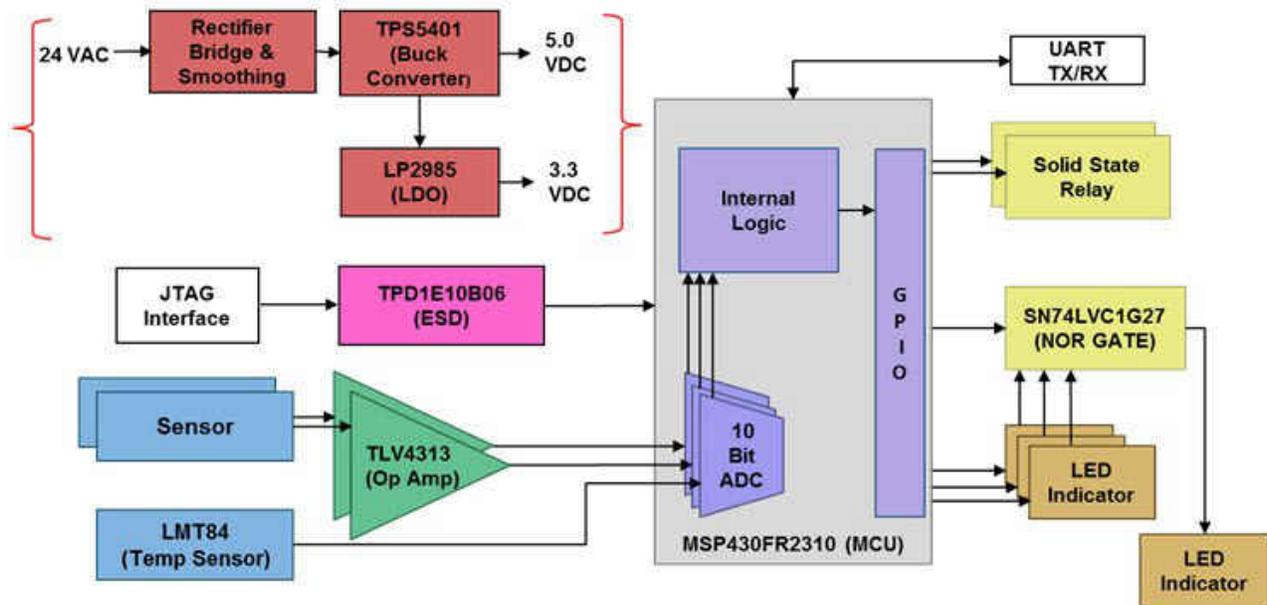
Figure 1. HVAC Coil Airflow Sensor System Block Diagram
