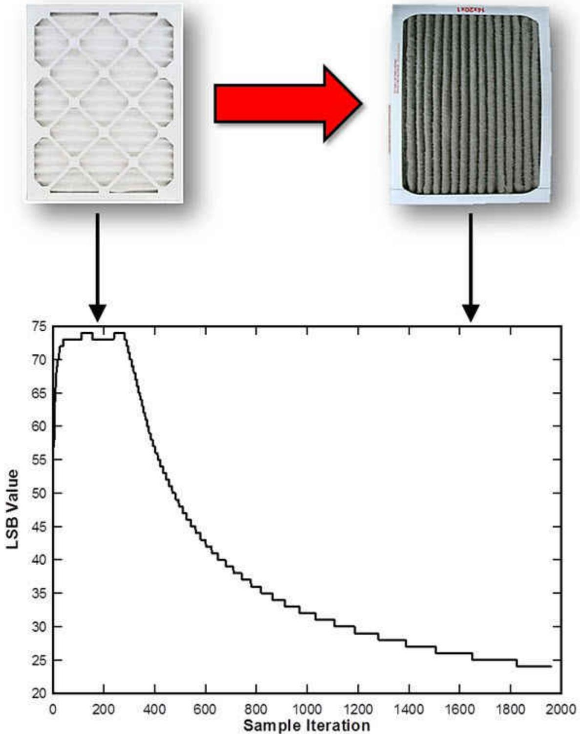
**Figure 2. TIDA-01070 HVAC Coil Airflow Sensor Reference Design Test Results**
