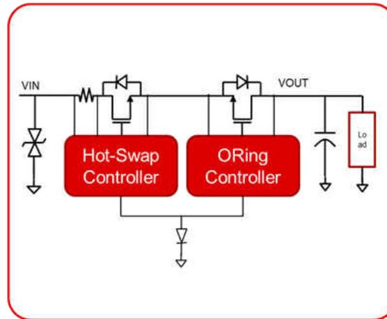
**Figure 2. Controller + MOSFET Protection Scheme**
