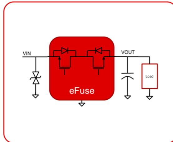
**Figure 3. Integrated Protection Scheme**
