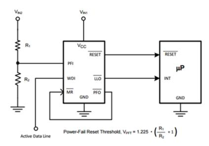
Figure 3. LM3710 Application Circuit
