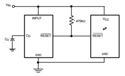
Figure 1. LM8365 Typical Application Circuit with Programmable Output Delay
