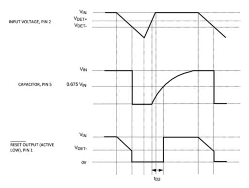
Figure 2. Timing Diagram for the LM8365
