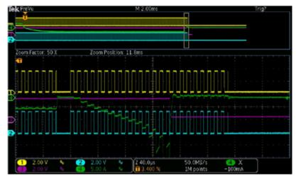
Figure 2. PWM Out-of-sync Leads to Inductor Current Surge (Blue: upper-FET PWM; Yellow: lower-FET PWM; Green: Inductor Current; Red: Fault-signal Triggering)
