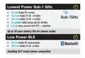
Figure 1. SimpleLink dual-band CC1350 wireless MCU power numbers
