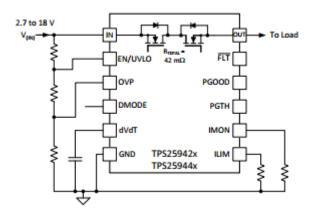
Figure 5. TPS25942 Simplified Schematic.
