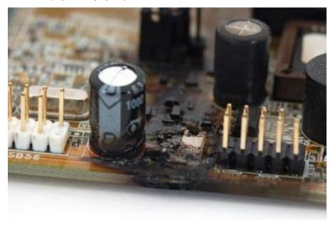
Figure 1. Damage to IC Due to over Voltage and over Current Events.
