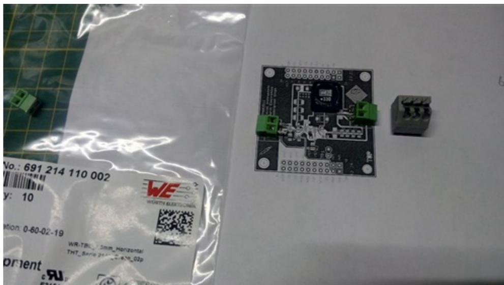
**Figure 3. Footprint Verification via 1:1 Paper Print of the Layout**
