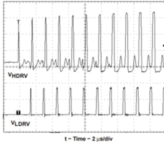
**Figure 4. MOSFET Drivers at Beginning of Soft Start under Pre-biased  $V_{OUT}$**
