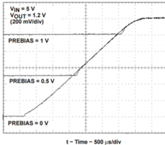
**Figure 5. Voltage Regulator Startup Waveforms under Pre-biased  $V_{OUT}$**
