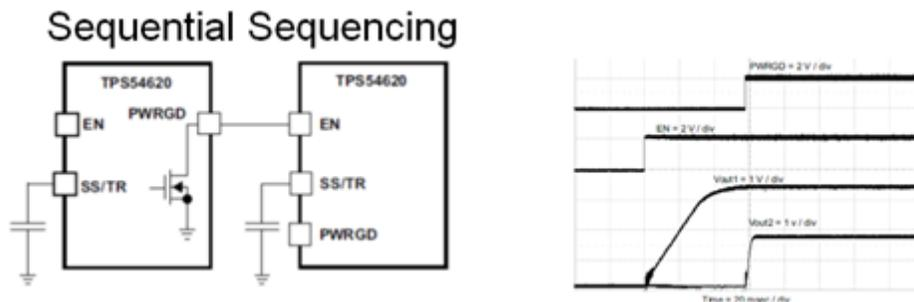
**Figure 1. Power Good and Enable for Power Sequencing**
