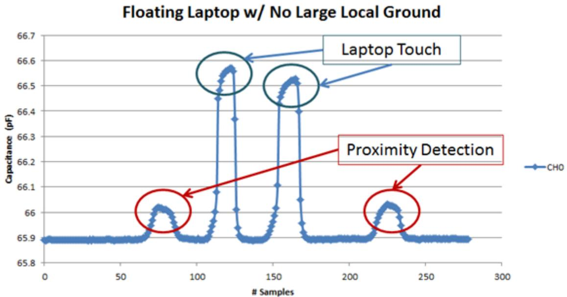
Figure 4. Capacitance Measurements of the System, with the Laptop Floating and No Large Local Ground
