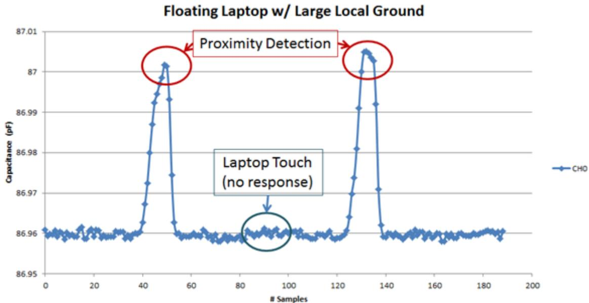
**Figure 5. Capacitance Measurements of the System with the Laptop Floating, but Also with a Large Local Ground Connected to the EVM**
