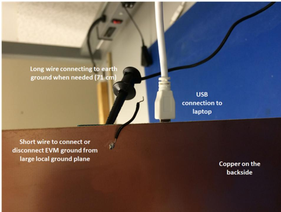
Figure 3. The Ground Plane Has Copper on the Backside (Seen Here) and FR-4 on the Topside (Seen in Figure 5)
