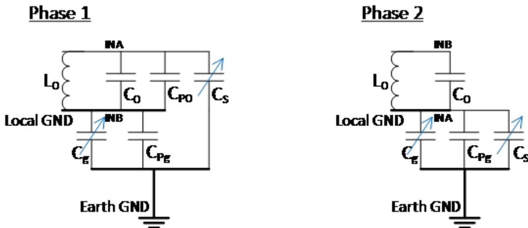
Figure 1. Simplified Circuit Model with the Resonator-based Capacitive Sensing Device Floating and a Large Local Ground Plane Nearby
