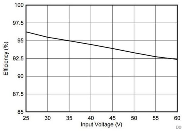
Figure 4. Efficiency vs. Input Voltage of Seven White LEDs at 1.5A (V<sub>OUT</sub> = 23V)
