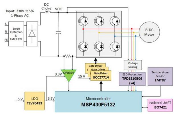
Figure 2. Block Diagram of a Simple 250W BLDC Three-phase Inverter Drive Stage for a 300V BLDC Motor
