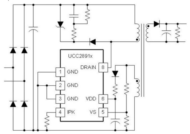
Figure 5. Flyback Switcher with Integrated 700V Switch and Low Standby Power Consumption
