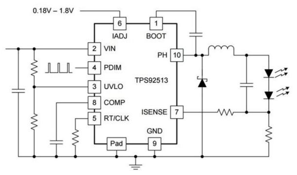
Figure 3. 1.5A Buck LED Driver with Integrated Analog Current Adjust
