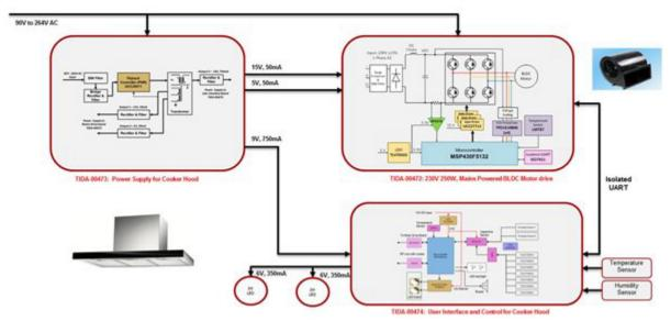
Figure 1. Cooker Hood System Block Diagram
