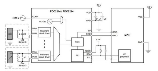
Figure 6. Application Schematic of FDC2214 Capacitance to Digital Converter
