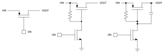
Figure 2. P-channel MOSFET (PMOS) Discrete Circuits
