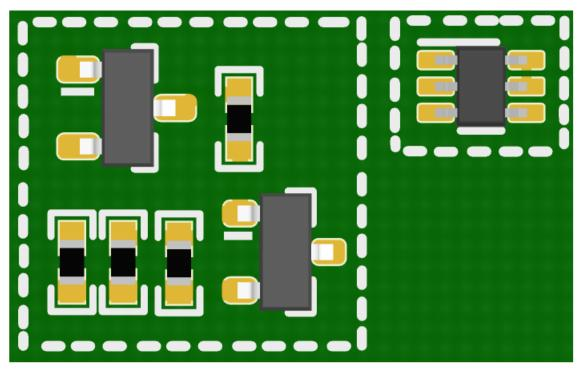
Figure 4. Size Comparison between the TPS22919 and an Equivalent Discrete Solution
