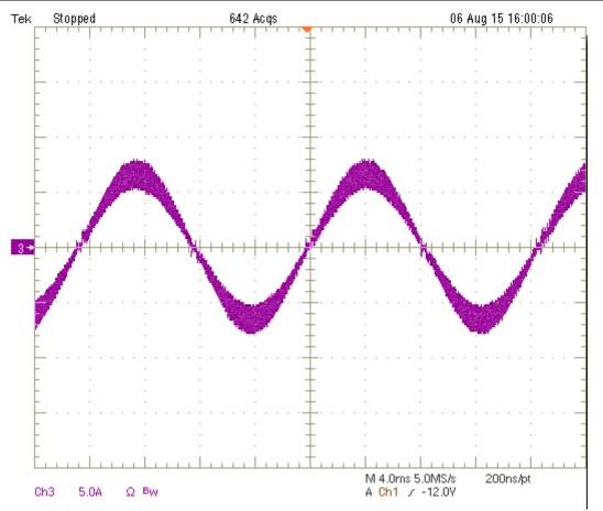
Figure 2. Current Waveform for a CCM Totem-pole PFC
