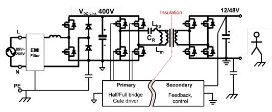
Figure 1. Simplified Circuit Diagram with Secondary-side Control
