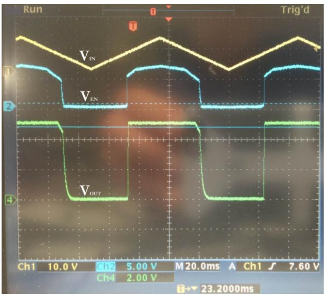
Figure 6. UVLO Controlled Waveforms
