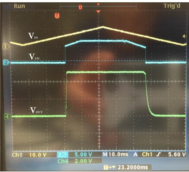
Figure 3. UVLO Controlled Waveforms
