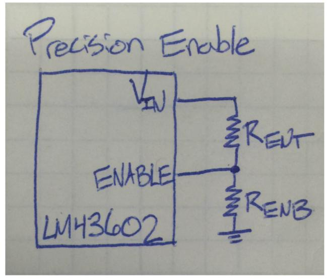
Figure 1. Simple Switcher <sup>®</sup> LM43602 Enable
