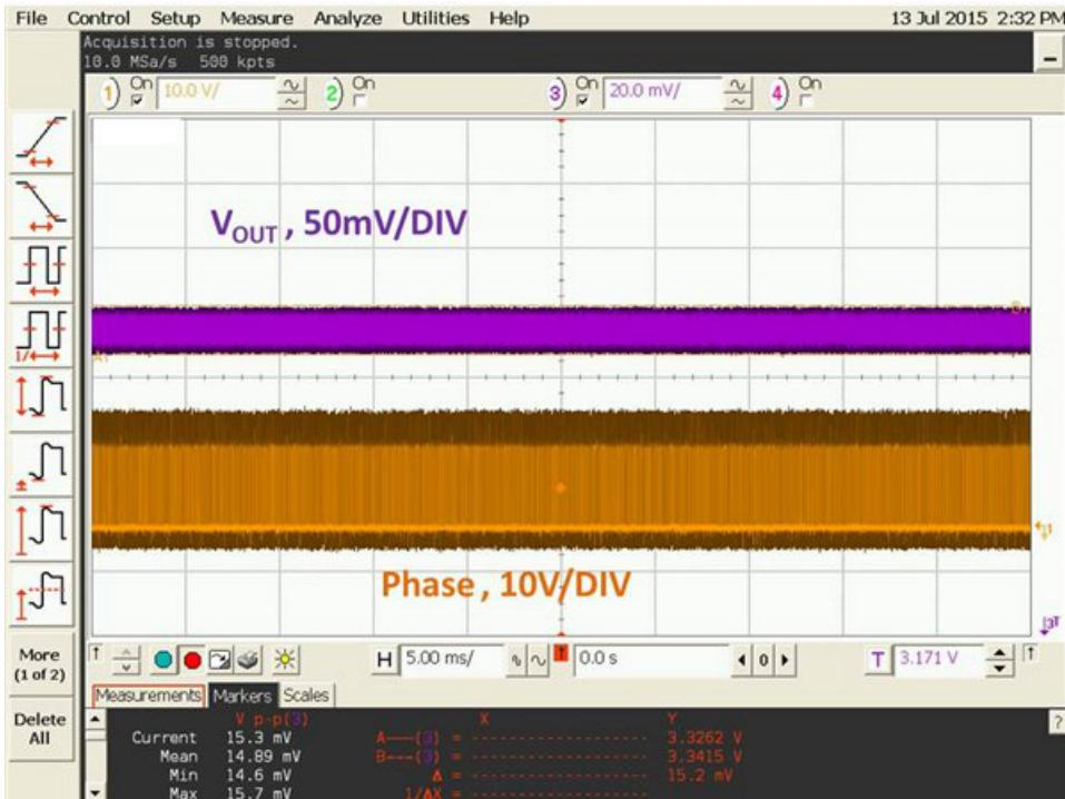
**Figure 9. Output ripple of the TPS53355 ( $V_{IN} = 12.6V$ ,  $I_o = 20A$ , oscilloscope in persistence mode)**
