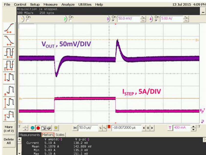
**Figure 8. Load-step transient response**
