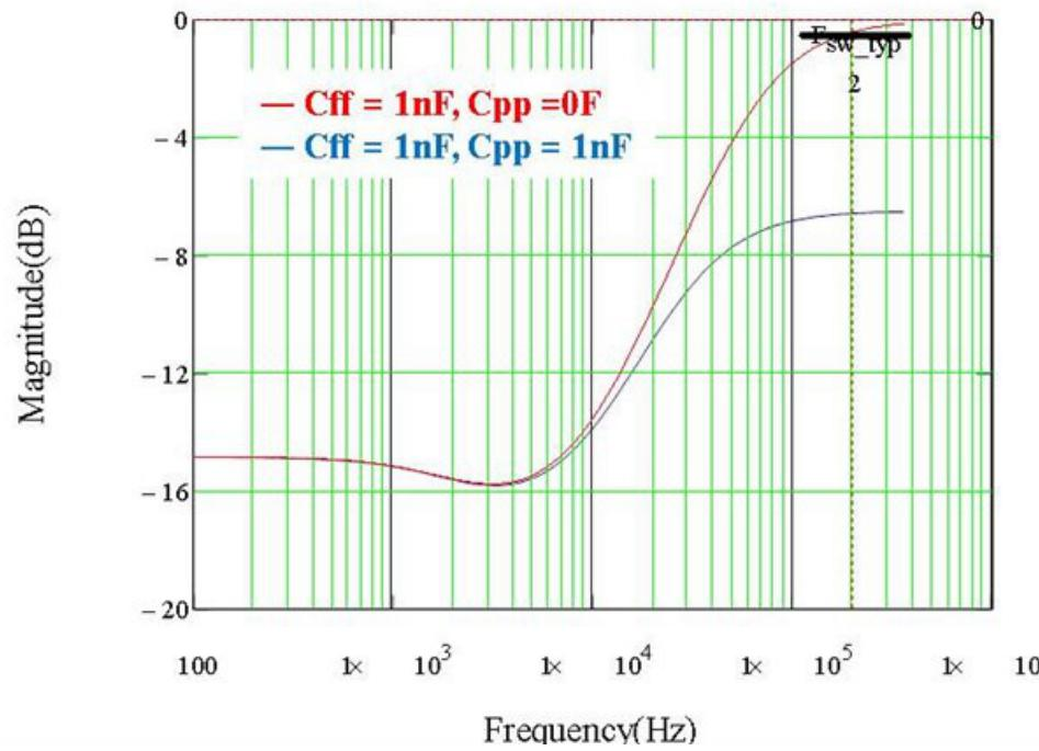
**Figure 4. Bode plots of transfer functions from  $V_{OUT}$  to FB with and without  $C_{pp}$**
