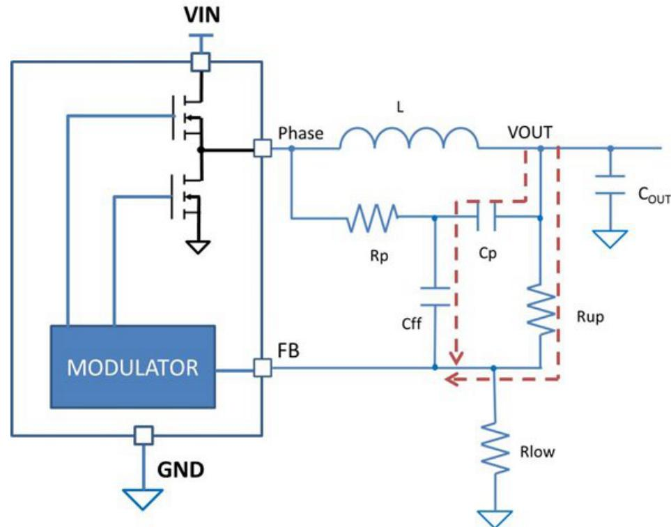
**Figure 3. Block diagram of a D-CAP regulator with a DCR injection circuit**
