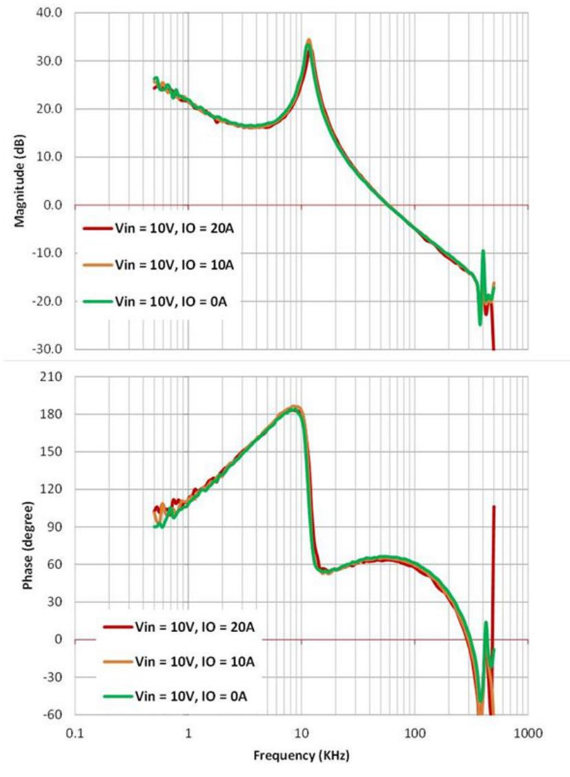
**Figure 7. Measured Bode plot of the TPS53355**
