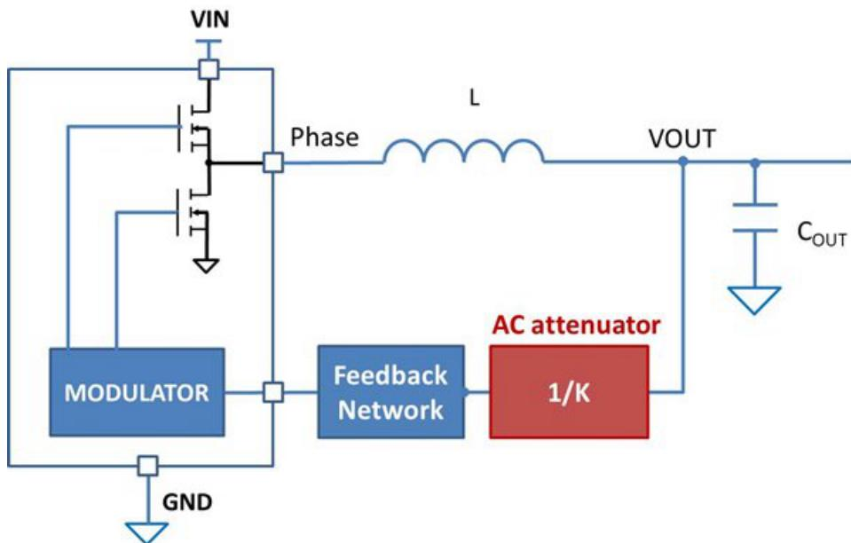
**Figure 1.** Buck converter block diagram with AC attenuator stage
