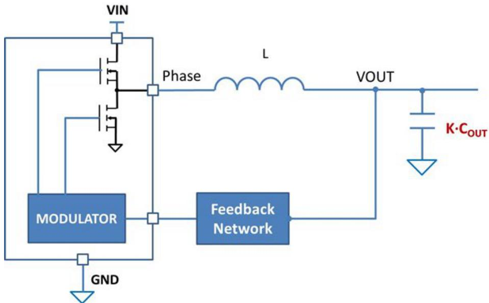
**Figure 2.** Equivalent block diagram with K times output capacitance
