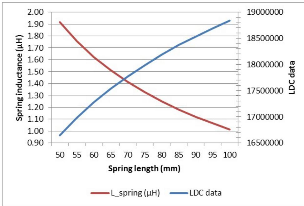
**Figure 4. LDC1612 Data and Spring Inductance versus Spring Length**
