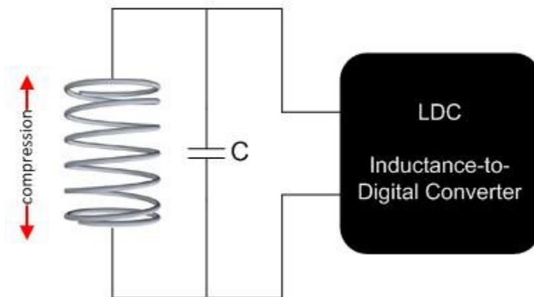
**Figure 1. Spring Used as a Sensor by an LDC**
