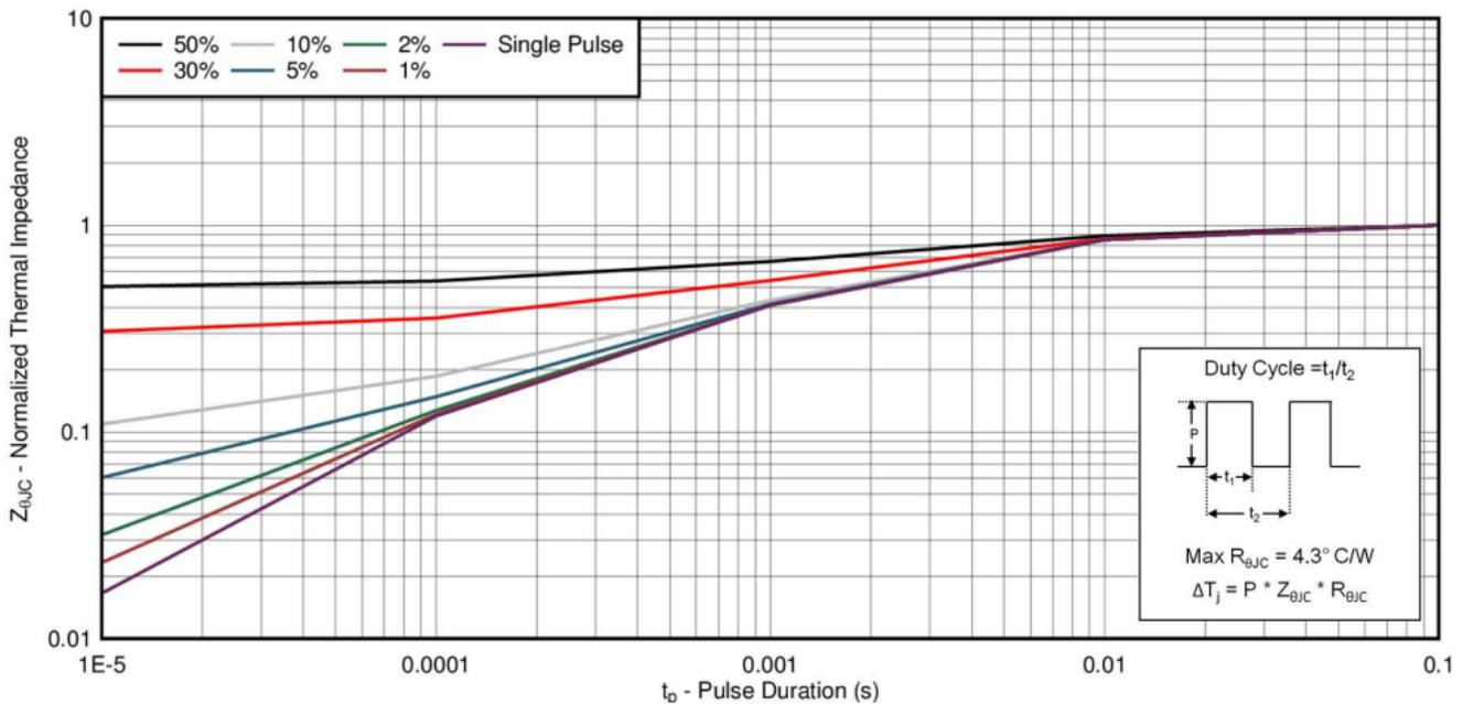
**Figure 1. CSD17579Q5A Normalized Transient Thermal Impedance Curve**
