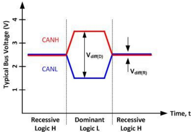
Figure 2. CAN Bus Signal Levels
