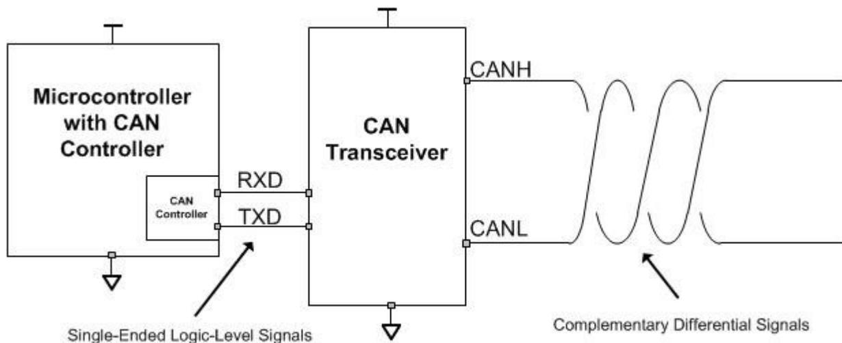
**Figure 1. CAN Controller and CAN Transceiver**
