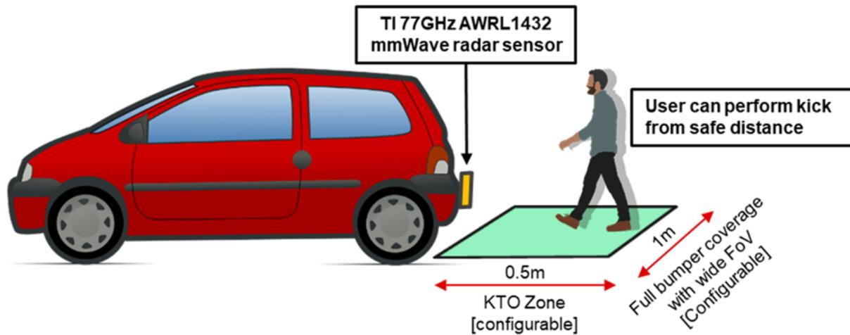
**Figure 1. An AWRL1432-based kick-to-open system implementation**
