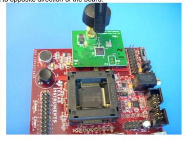
Now you have completely programmed host processor and network processor on MSP430F5438 experimenter board.
