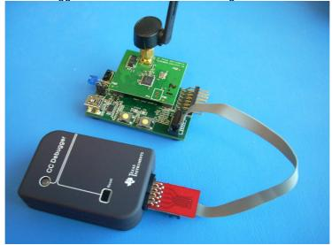
Connect USB cable from PC to the RemoTl Target Board.
