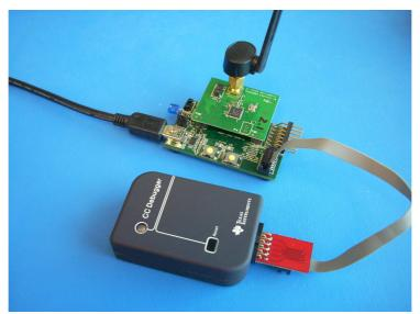
Connect USB cable from PC to CC debugger. CC debugger should turn on green LED. If it turned on RED instead, preset RESET button on CC debugger. If the LED still remains red, remove the USB cables and connect the cables again.
