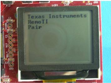
Perform pairing by pressing "S1" key once. LED1 on MSP experimenter board will blink till the pairing completes or fails. Operate the target emulator to pair the device. Pairing uses CERC push button pairing protocol.
