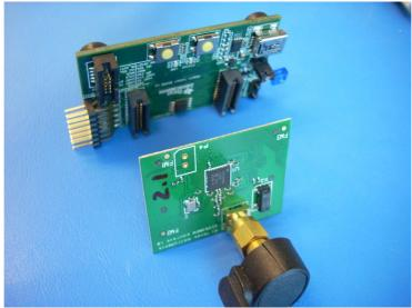
• Install the extra CC2530EM module into the RemoTI Target Board.
