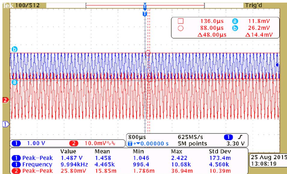
**Figure 20. DC-DC PSRR Measurement Result, Frequency 10 kHz**
