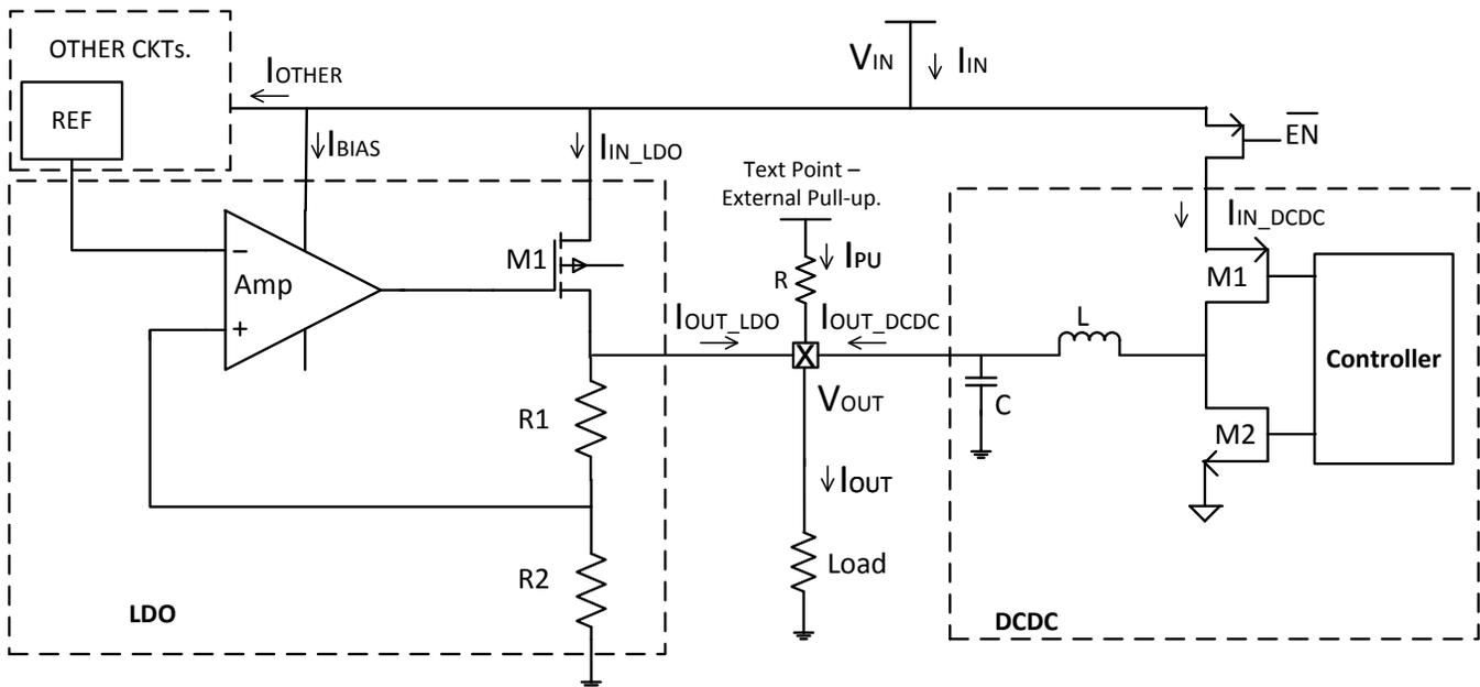
**Figure 6. DC-DC and LDO Configuration in CC2640**
