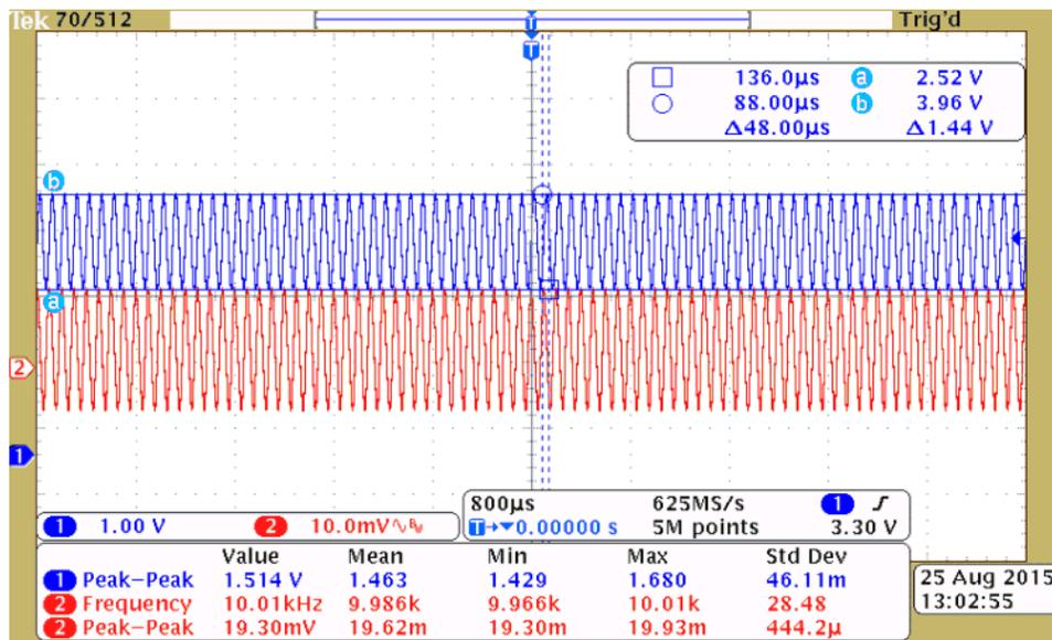
Figure 19. LDO PSRR Measurement Result, Frequency 10 kHz
