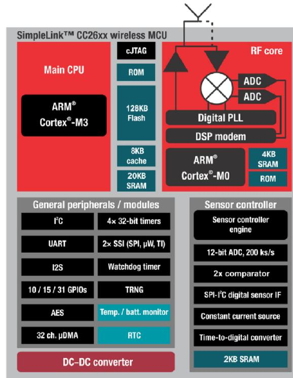
**Figure 1. CC2640 Block Diagram**
