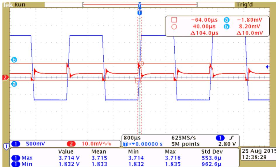
Figure 15. LDO Line Regulation Measurement Result
