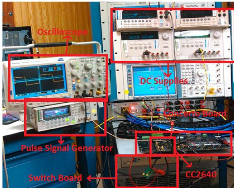
Figure 11. Load Regulation Setup Picture
