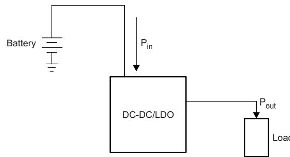
Figure 5. Basic Regulator Configuration
