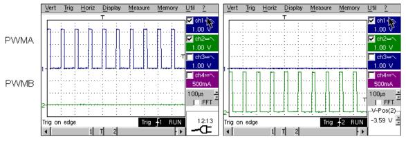
Figure 7. PWMA and PWMB for VRef1 = 0.25 and -0.25
