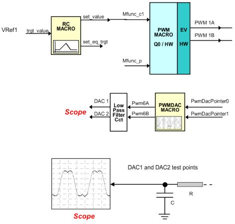
(1) Level 1 verifies the target independent modules, duty cycles, and PWM updates. The motors are disconnected at this level.
