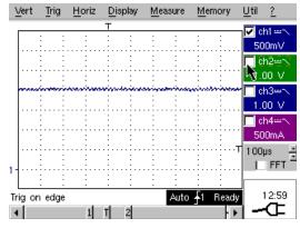
Figure 8. PWM DAC2 output for VRef1 = 0.25
