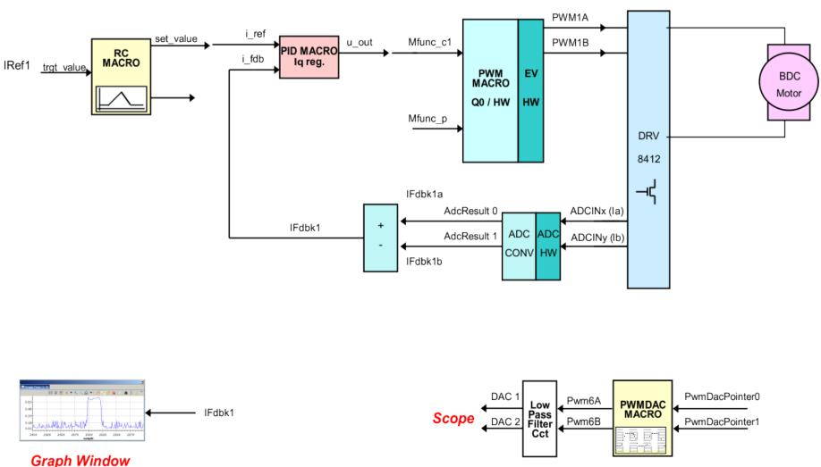
Level 3 verifies the close-loop current regulation performed by pid\_i module
