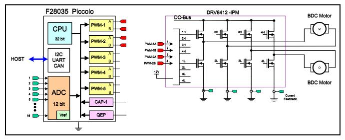
Figure 1. Dual-Axis, Brushed DC Motor Drive
