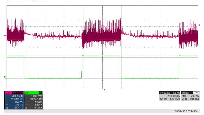
Figure 14. 230 VAC Load Transient
