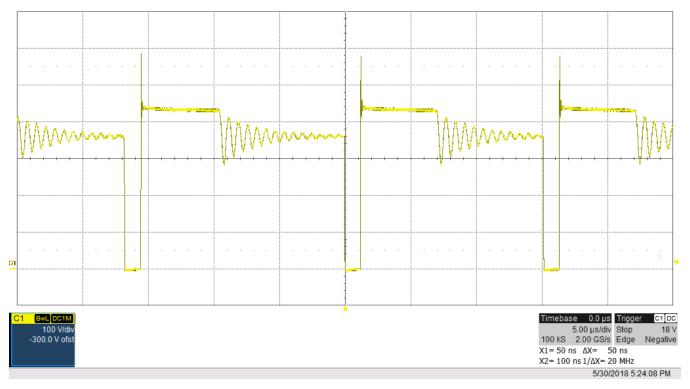
Figure 8. V<sub>ps</sub> of Primary Side MOSFET (Q1)
