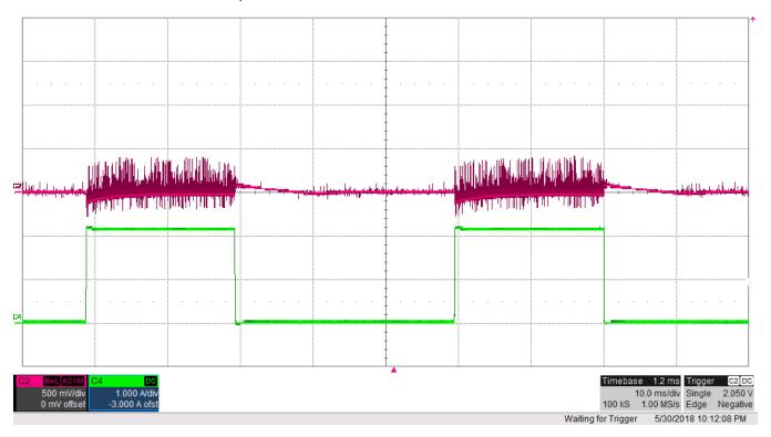
Figure 15. 120 VAC Load Transient
