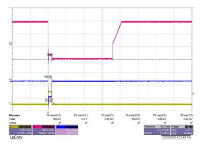
Figure 15.  $V_{IN}$  = 12 V,  $I_{OUT}$  = 160 A, Short Circuit and Recovery
