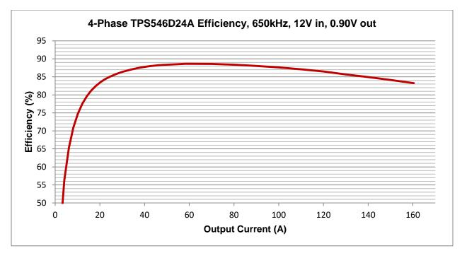
Figure 1. Efficiency vs. IOUT
