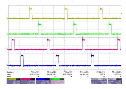
Figure 10. Switch Node Waveforms (No Load)
