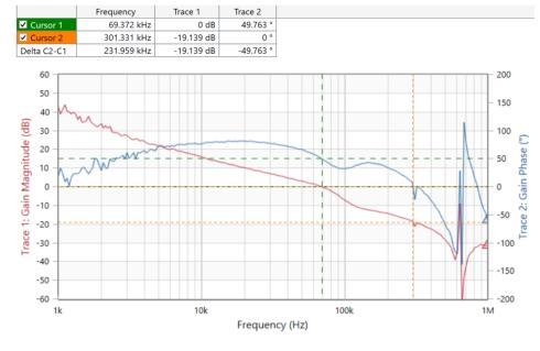
The crossover frequency is 69.372 kHz. The gain margin is 19.139 dB and the phase margin is 49.763°.
