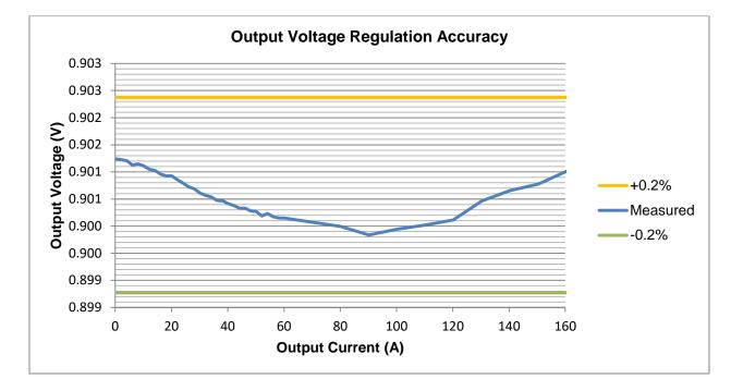
The output voltage is regulated to within 0.11% of the nominal 0.9V.
