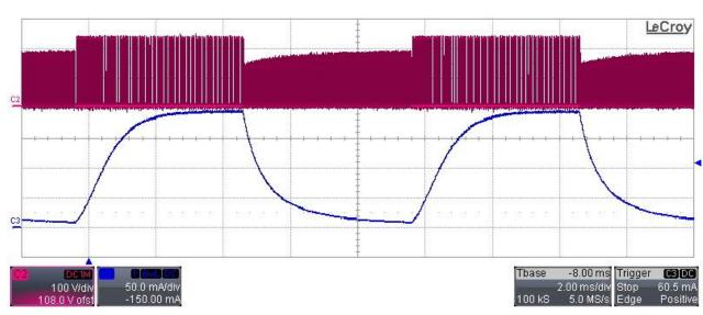
Ch.2: Switch-node (Drain of Q1) (100V/div, 2msec/div, no BWL) Ch.3: Output current ripple (LED current) (50mA/div, 20 MHz BWL)
