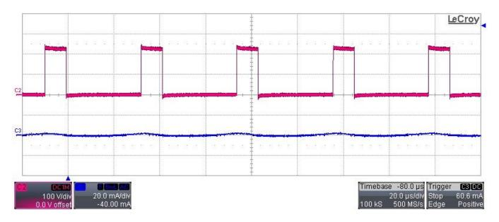
Ch.2: Switch-node (Drain of Q1) (100V/div, 20usec/div, no BWL) Ch.3: Output current ripple (LED current) (20mA/div, AC coupling, 20 MHz BWL)
