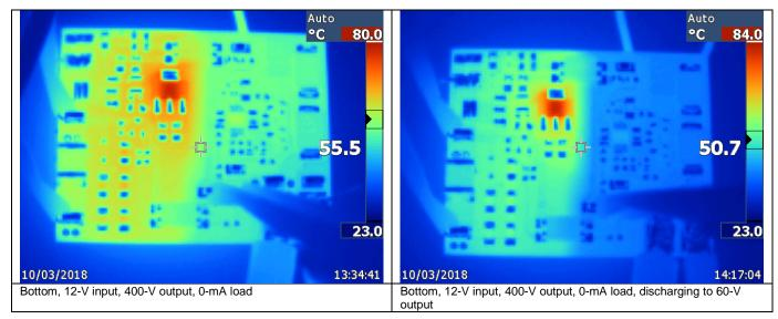
The hot spot at no load is the secondary-side high voltage standoff transistor. The maximum shunt regulator current is set for 2 mA, resulting in 0.8 W of power dissipation at 400 V out.
