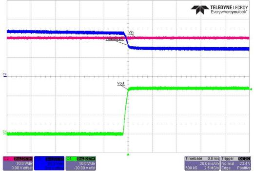
Input Voltage = 20VDC Load current = 0A
