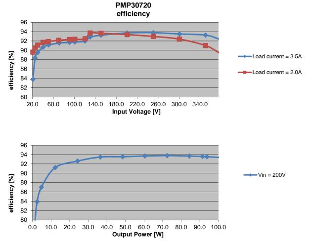
The NTC RT100 was shorted for the efficiency measurements.
