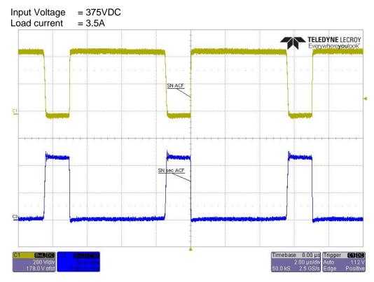
Channel 1: Switch Node active clamp flyback (Q2) Channel 2: Secondary Side Switch Node (Q3)
