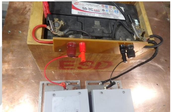
Picture for battery & LISN grounding
