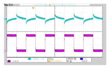
Figure 3-9. 13.5-V Input, 0-A to 2.4-A Output; CH2: V<sub>BUS AC</sub>, CH3: I<sub>BUS</sub>
