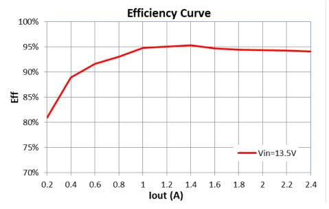
Figure 2-1. Efficiency Graph
