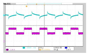
Figure 3-8. 13.5-V Input, 1.5-A to 2.4-A Output; CH2: V<sub>BUS\_AC</sub>, CH3: I<sub>BUS</sub>
