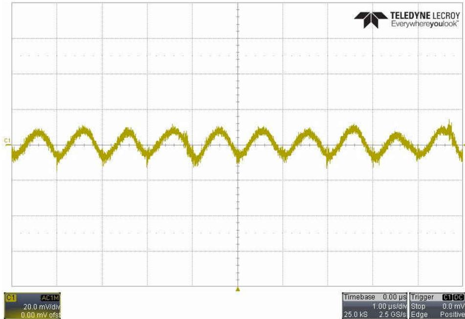
Figure 3-3. Output Voltage Ripple of LS Rail
