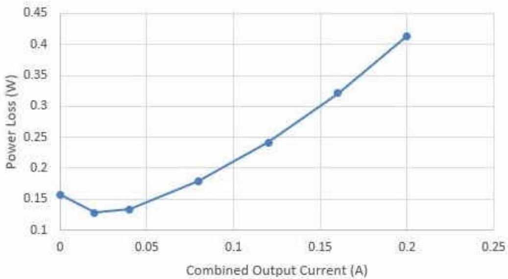
**Figure 2-3. Power Loss Graph – HS and LS Rail Current Split Evenly**
