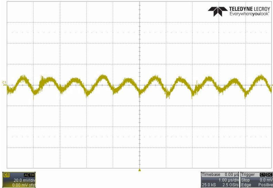
Figure 3-2. Output Voltage Ripple of HS Rail
