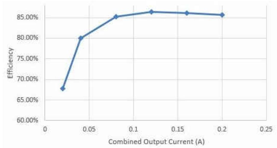
Figure 2-2. Efficiency Graph – HS and LS Rail Current Split Evenly
