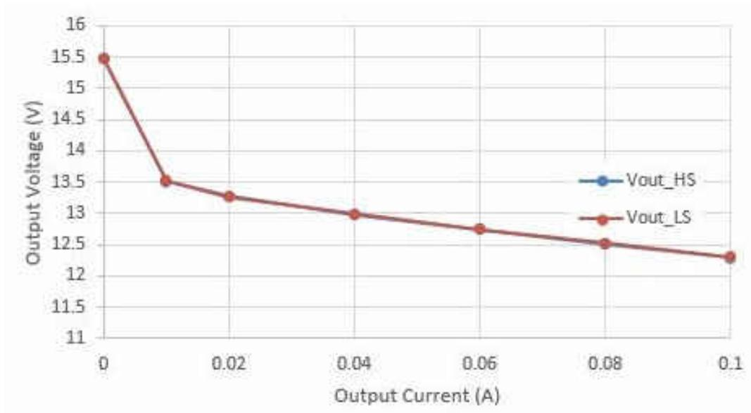
Figure 2-1. Open Loop Output Voltage vs Output Current
