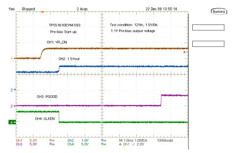
Note: The unit could not start up if the pre-bias voltage is higher than 1.1V
