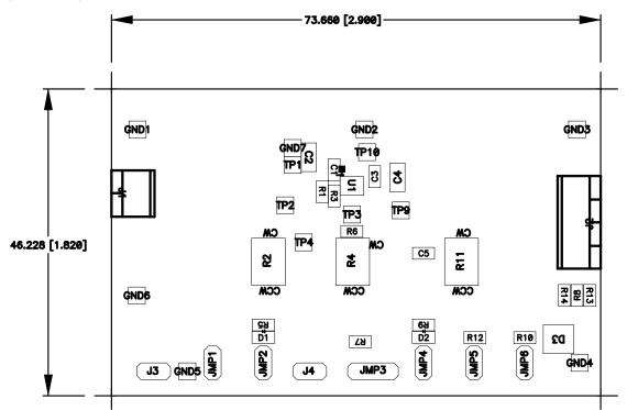
Figure 3. Assembly Layer
