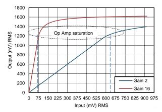
Figure 9. PGA116, Saturation
