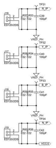
**Figure 4. Current Inputs Schematics**
