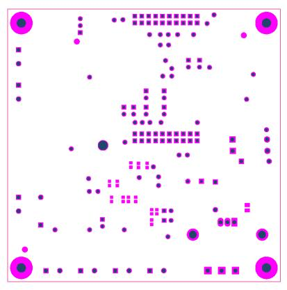
Figure 30. Bottom Solder Mask
