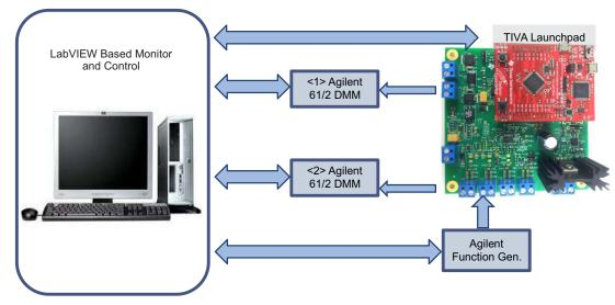
Figure 8. TIDA-00128 Test Setup
