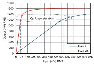
Figure 10. PGA117, Saturation
