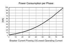
Figure 6. Typical Power Consumption for Current/Lowest Operating Current
