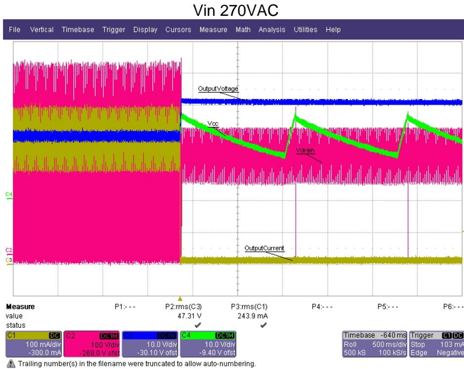
When an Open LED condition is detected, the device is not turned off. It continuously checks if the output has been brought under limits
