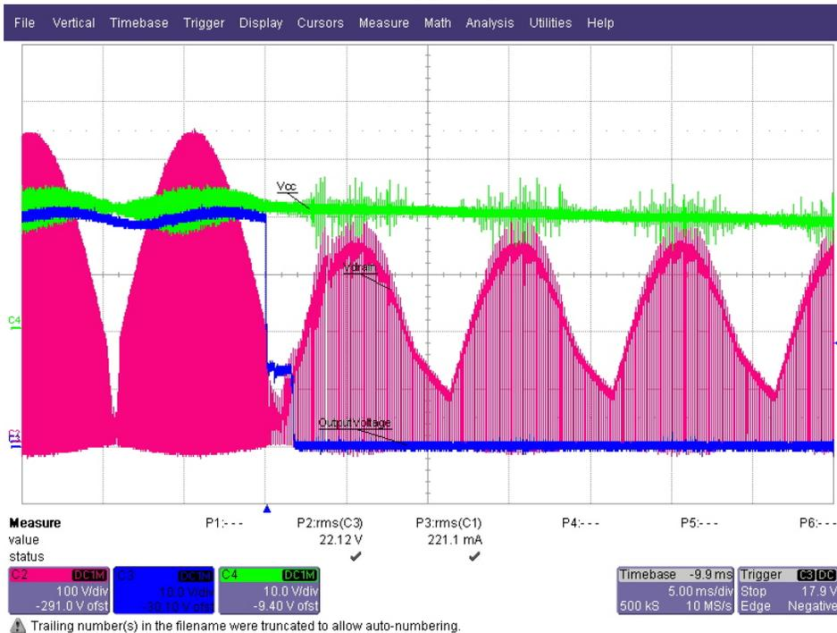
When a short circuit condition occurs, the controller goes into a hiccup mode and reverts back once the short condition is removed.
