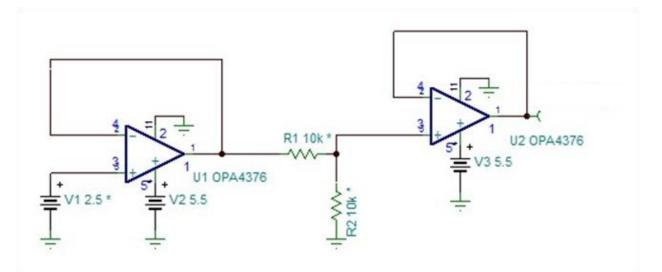
Figure 6: TINA-TI schematic to calculate offset error
