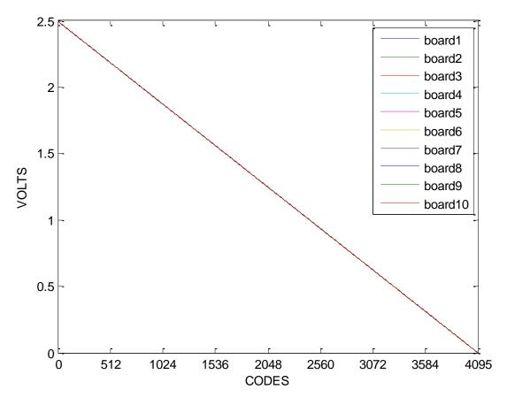
Figure 9: Measured transfer function
