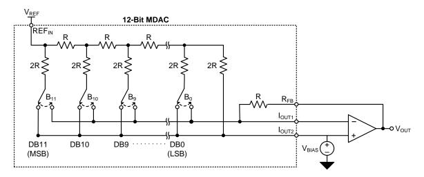
Figure 4: MDAC with offset voltage
