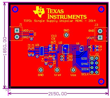
Figure 7: PCB Layout, Top Layer
