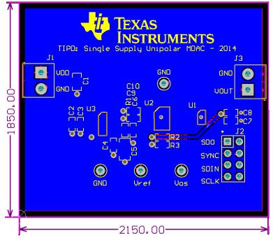
Figure 8: PCB Layout, Bottom Layer
