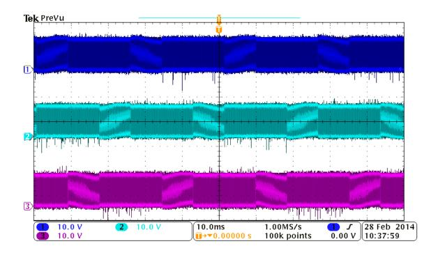
Figure 1 Motor phase voltages (A,B,C) during operation
