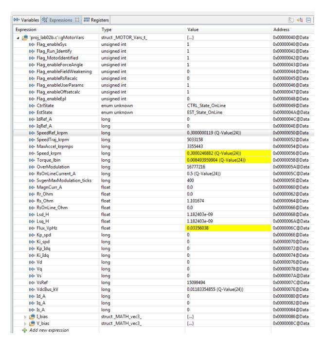
User Interface for Motor Variables to control BLDC
