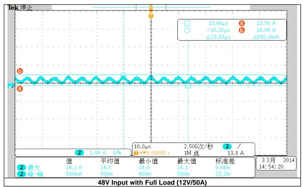
Test point is between the DC Power Supply and the input capacitors.
