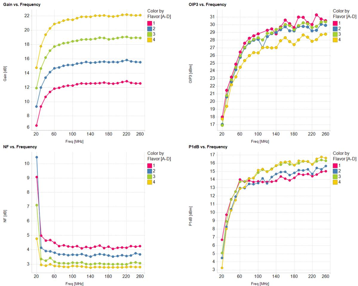
**Figure 2: Low Frequency Performance with Nominal RF Component Values**
