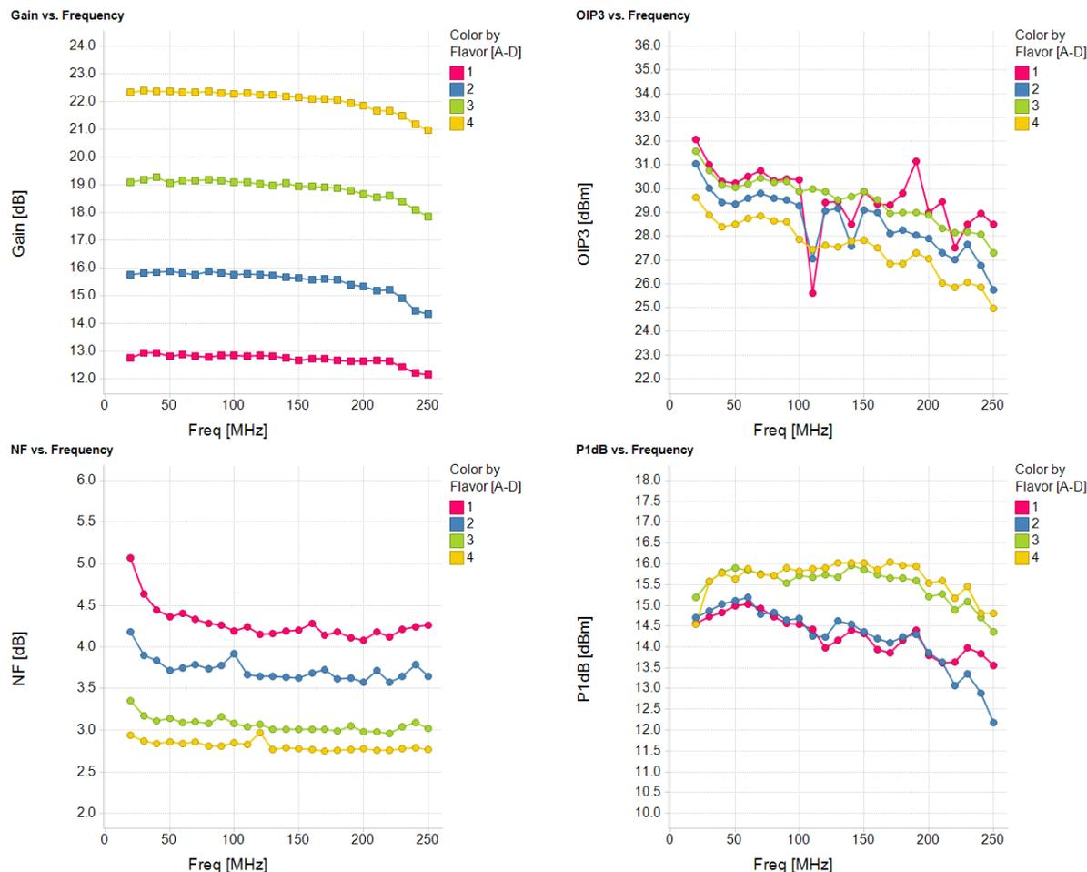
**Figure 3: Low Frequency Performance with LF Optimized RF Components**
