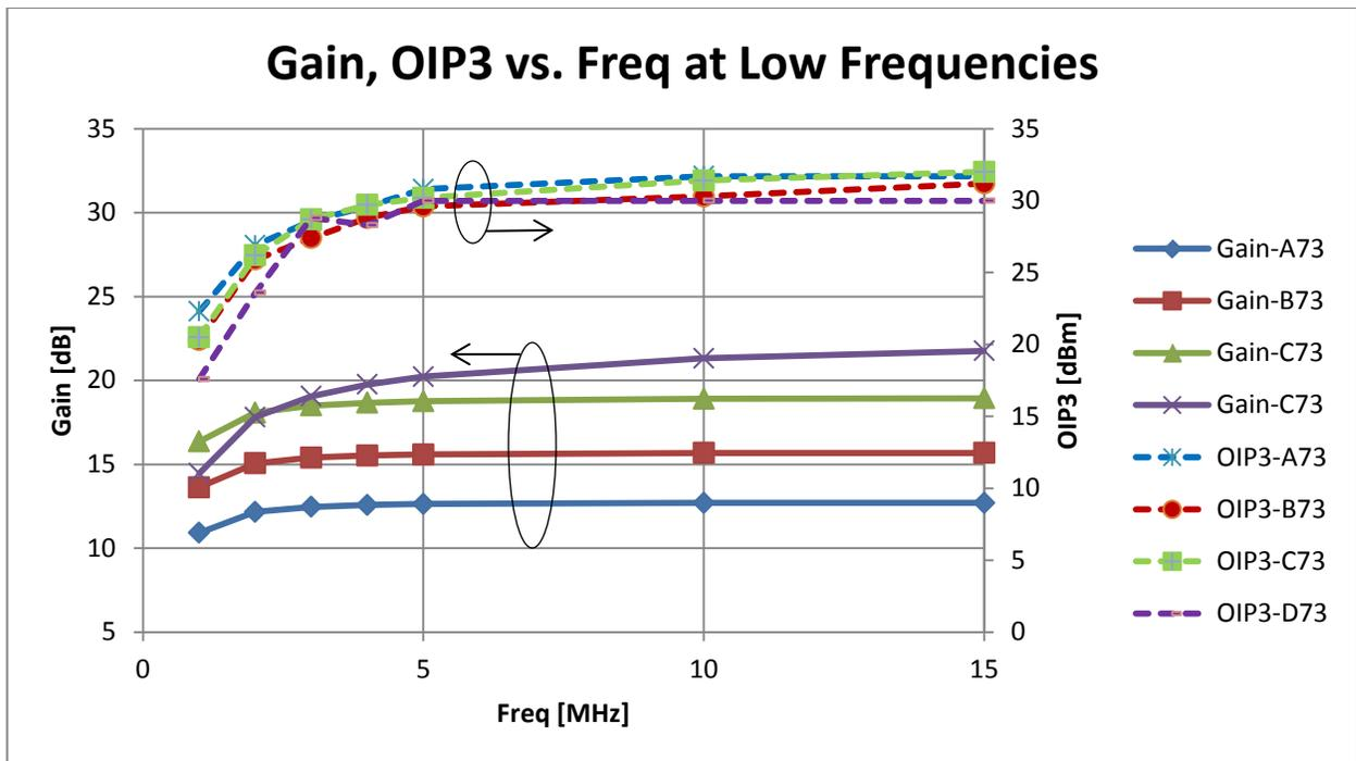
Figure 4: Gain and OIP3 Response down to 1 MHz
