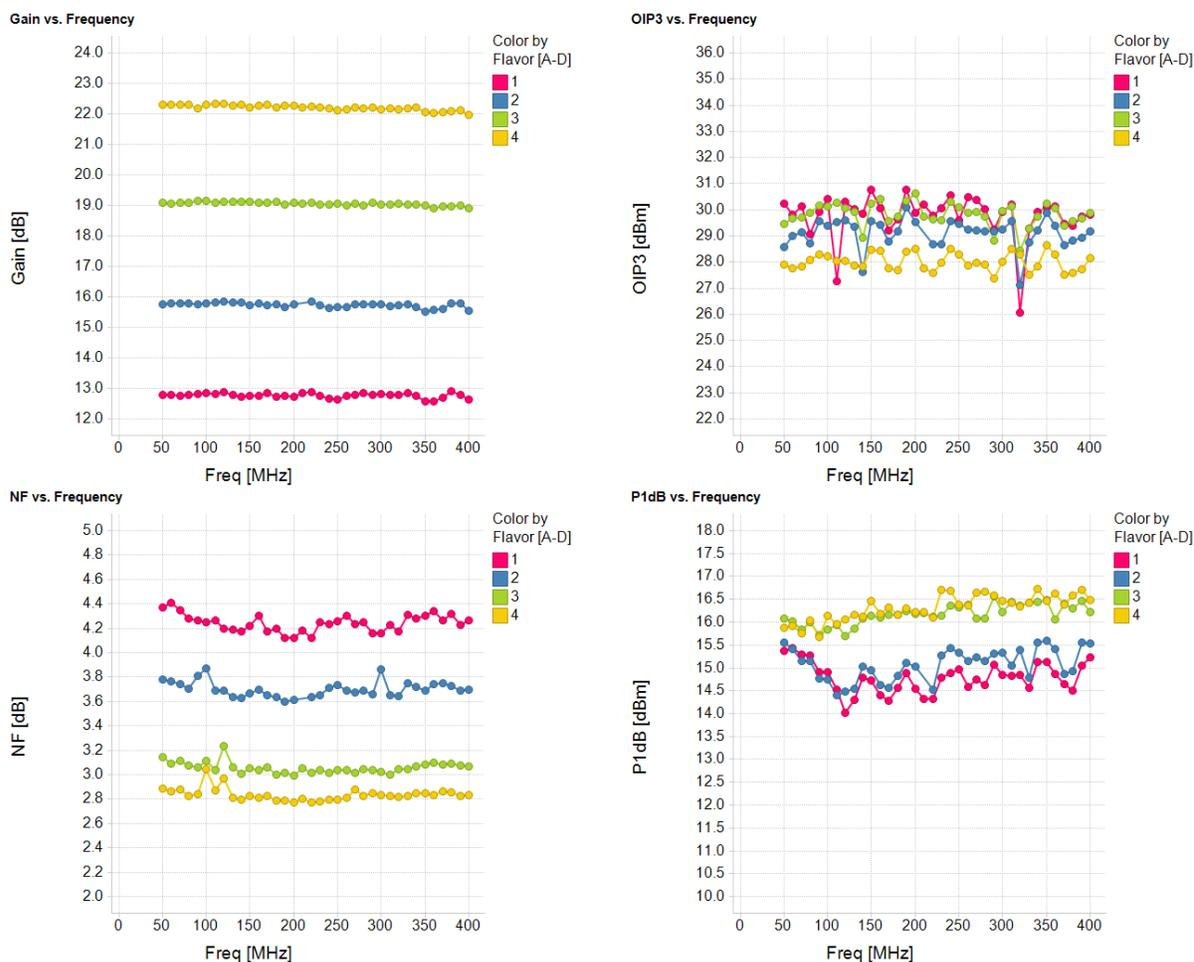
**Figure 5: Low Frequency Performance with IF Optimized RF Components**
