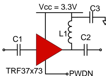
**Figure 1: Application Schematic**
