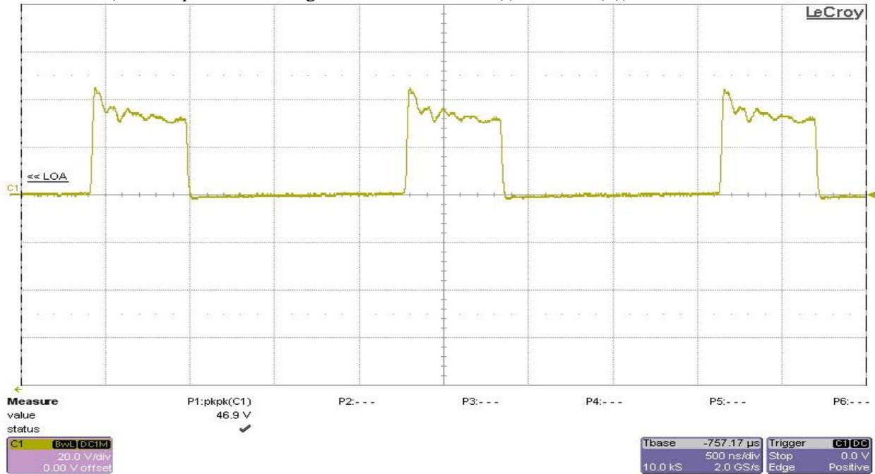
Test condition: The input voltage was set at 32V, and four outputs were set at full load of 75mA.
