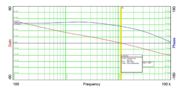
The plot below shows the converter's gain and phase margin for an LED current of 0.5A.
