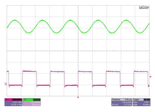
The waveforms below show the switch node voltage (RED) at TP2 and the LED current (GREEN). The input voltage is 12V and the LED output is regulated to 0.5A. (5V/DIV, 100mA/DIV, 1uS/DIV)
