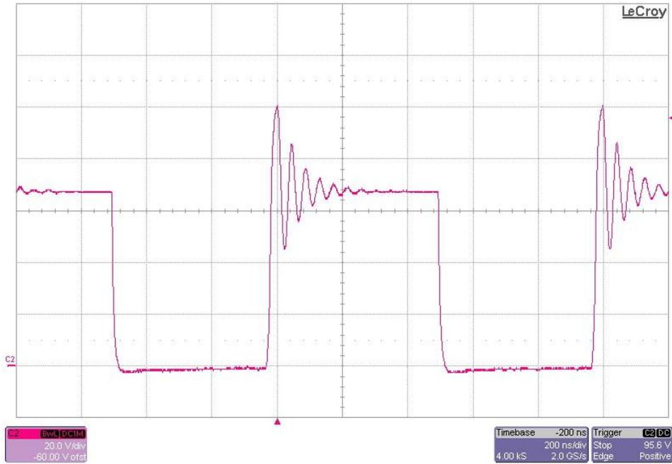
The photo below shows the FET switching voltage (TP5) for an input voltage of 57V and a 1A load. (20V/DIV, 200ns/DIV)
