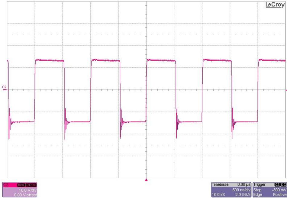
The photo below shows the 12V transformer secondary voltage. The input voltage was set to 57V with a 1A load. (10V/DIV, 500nS/DIV)
