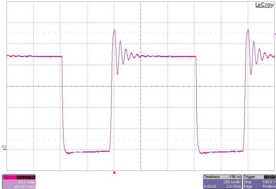
The photo below shows the FET switching voltage (TP5) for an input voltage of 36V and a 0.09A load. The converter has just transitioned to DCM at this load. (20V/DIV, 200nS/DIV)
