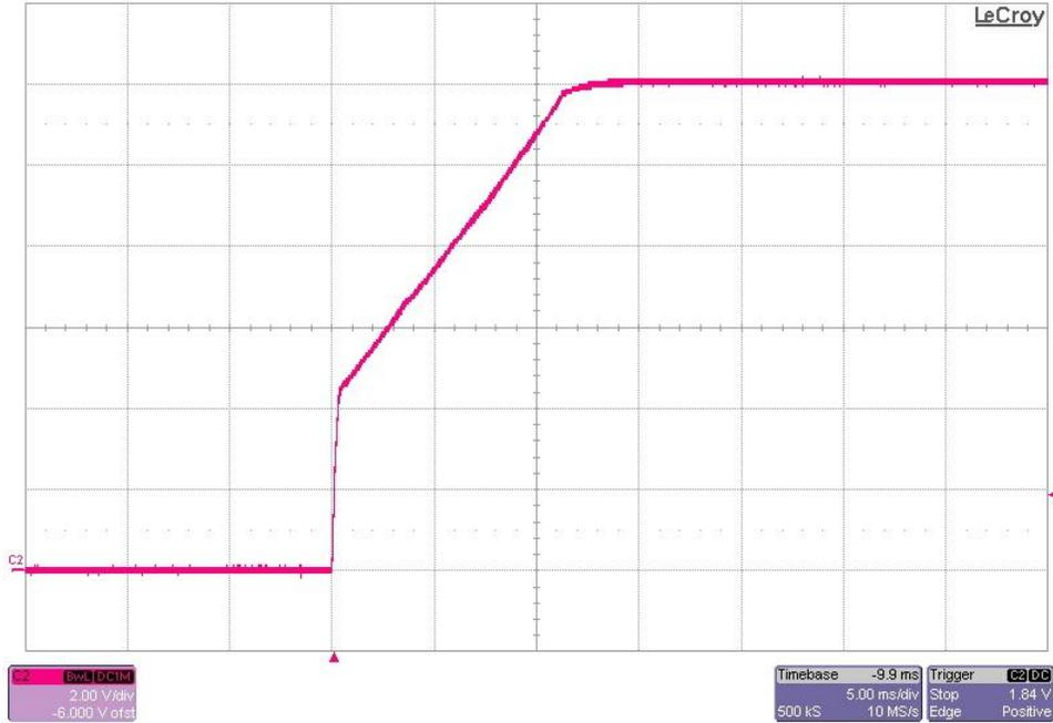
The photo below shows the output voltage startup waveform after the application of 48V in. The 12V output was loaded to 1A and operating at 1MHz. (2V/DIV, 5mS/DIV)
