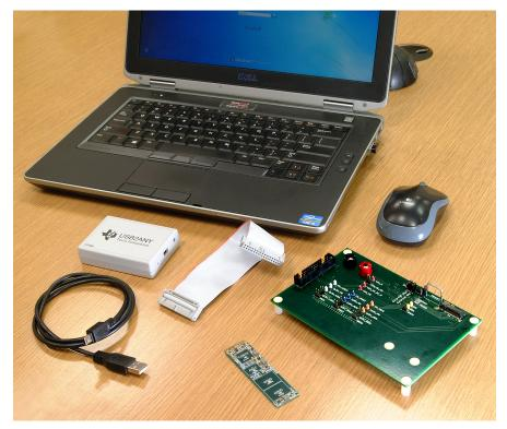
Figure 17. SSD Power Delivery System and Required Components
