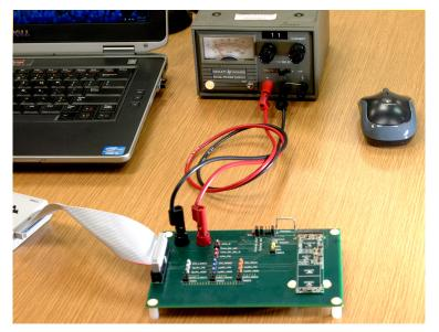
Figure 28. Auxiliary Power Supply Connected to Interposer Board
